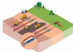
Installing underground cable – cut and fill method. Click image to enlarge
